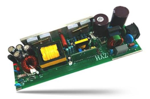
Max.350W power supply, with easy switch of AC220V/AC110V, universal supply for different countries.
